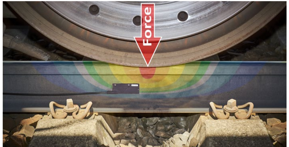
The strain applied to the Lite4ce™ sensor
